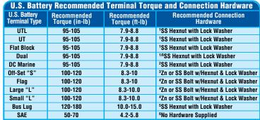
Proper connection is to position a lock washer between the nut and the connector (never between the connector and lead terminal) and apply the recommended torque or enough torque to completely compress the lock washer without deforming the lead terminal.
